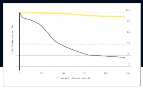
PA6-based warp-knitted fabrics containing either 20% XLANCE or 20% Spandex dipped in a 4-ppm-chlorine solution while under continuous dynamic stretch for over 200h.
