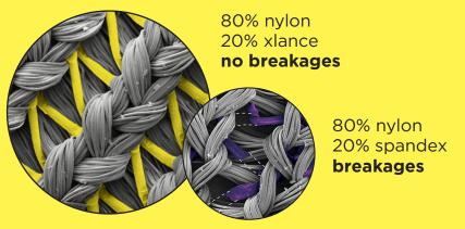
Images of competition garments containing either XLANCE or spandex after 5 months of swimwear test: XLANCE remains fully intact while spandex fiber is broken and fragmented by oxidative degradation.
